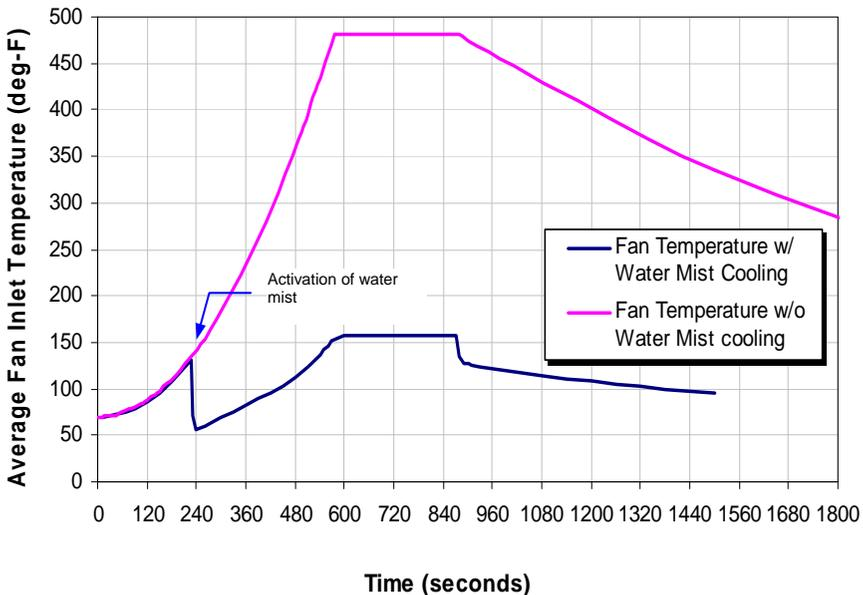
Figure 7. Resultant effect of evaporative cooling with water mist on air temperature reduction in exhaust chamber.
