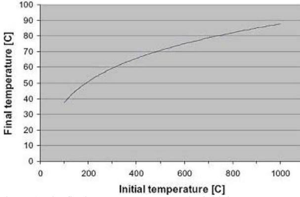
Figure 1. The final gas temperature vs. the initial gas temperature, assuming sufficient amount of water mist is applied.
