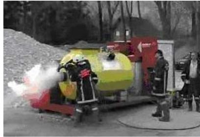
Figure 8. Cooling effect of water mist system test results (left: Tunnel fire test by Marioff; right: FOGTEC gas cooling test).
