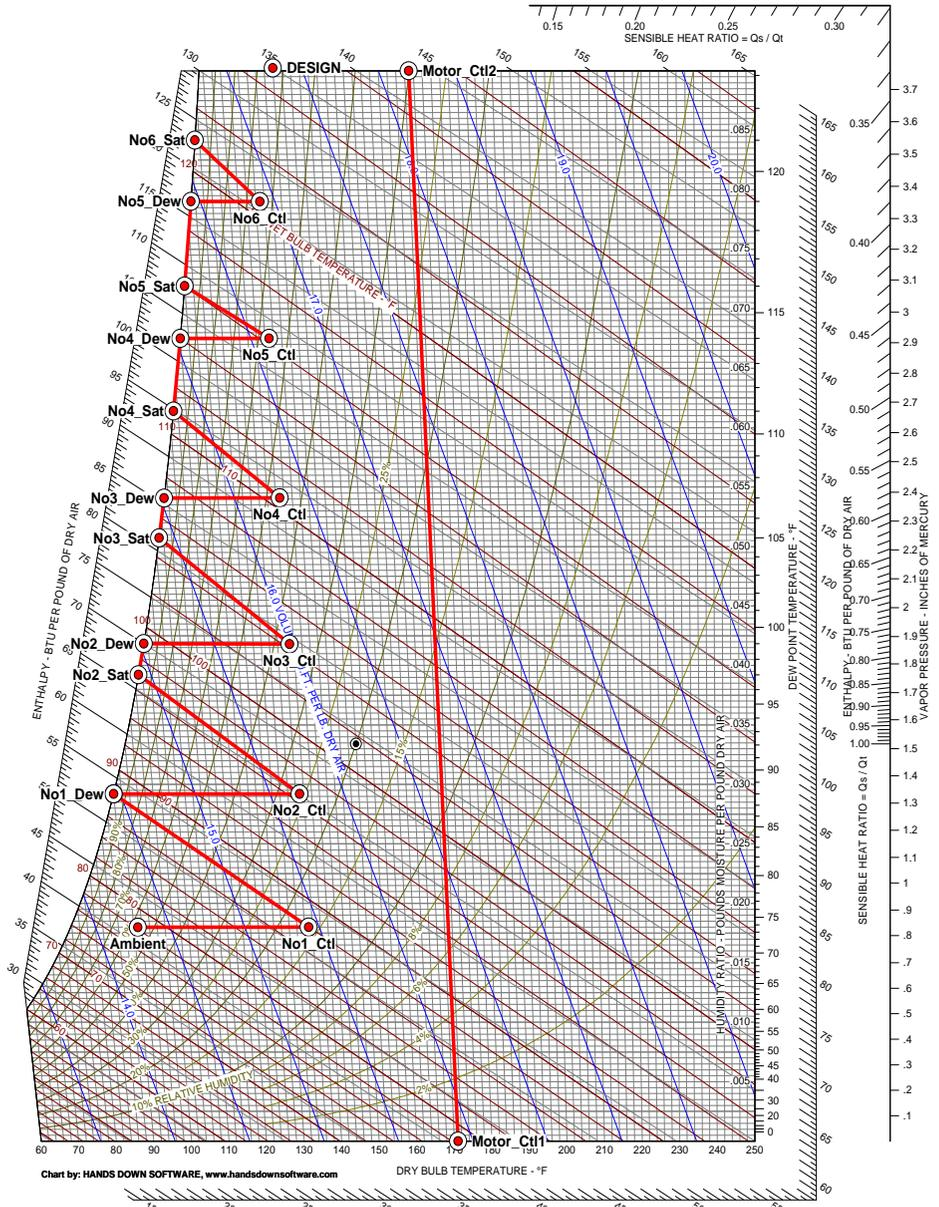
Figure 3. Psychrometric Chart for exhaust chamber evaporative cooling based on individual nozzle activation control system.
