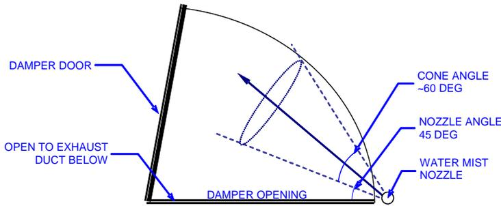
Figure 4. Inlet duct opening and angle of water mist nozzle supply.
