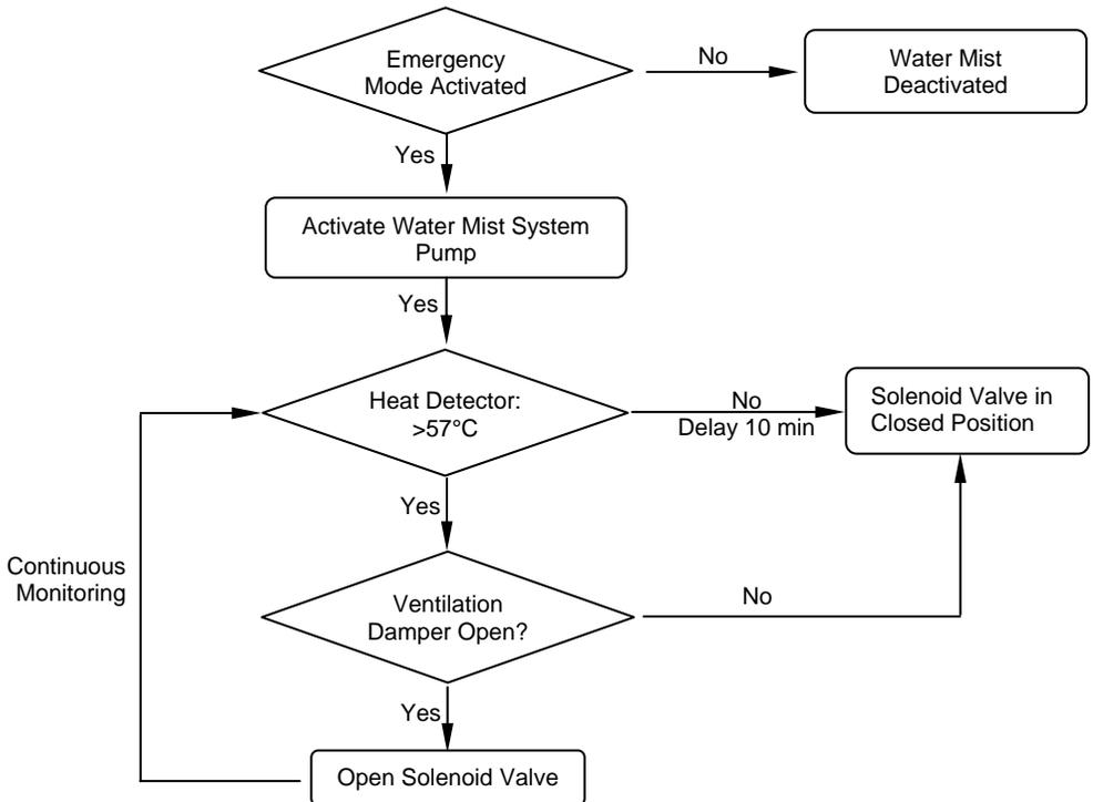
Figure 2. Typical control diagram for water mist exhaust chamber cooling system.
