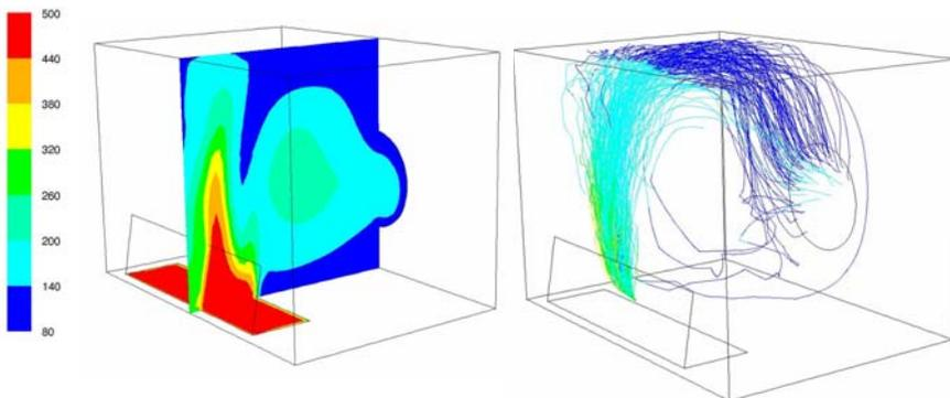
Figure 6. CFD Analysis Results – Air Temperature and Water Mist Particles Trajectory.
