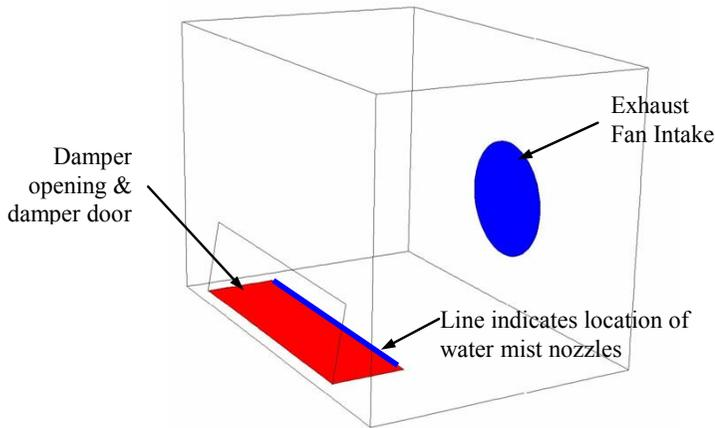
Figure 5 Simplified CFD Model of exhaust fan chamber.
