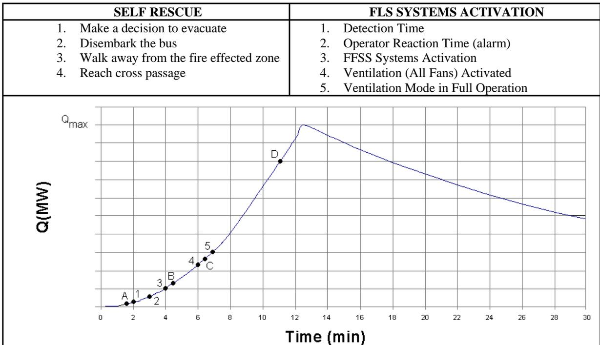
Figure 3 Example of project established time-of-tenability curve
