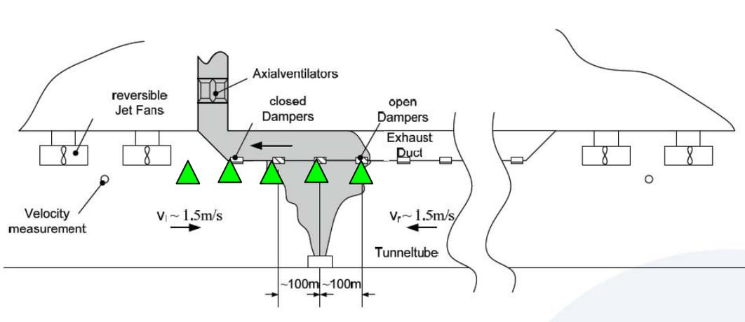
Figure 2 Single Point Extractions with Fixed Fire Suppression System
