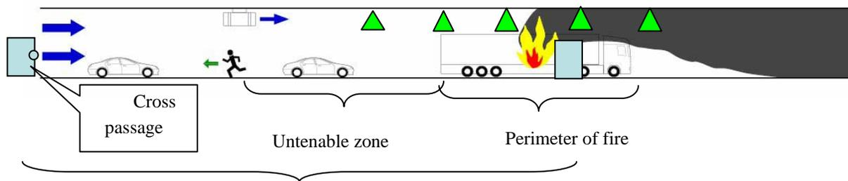
Figure 1 Longitudinal Ventilation with Fixed Fire Suppression System
