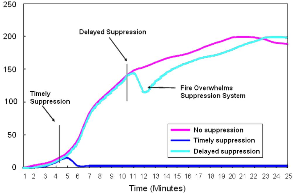
Figure 4 Schematic Effect of Suppression on Heat Release Rate
